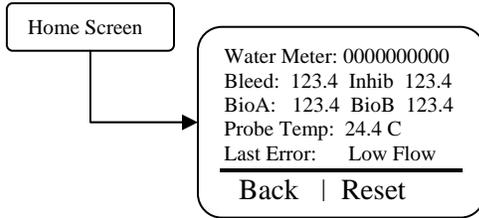
This screen shows the real-time data relating to the controller. This screen can be used to log the amount of time a particular output was energized since it was last reset.
