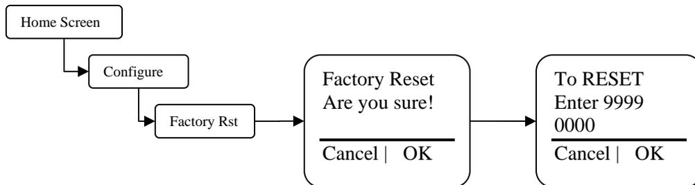
Use this function to reset the controller back to the factory defaults.
