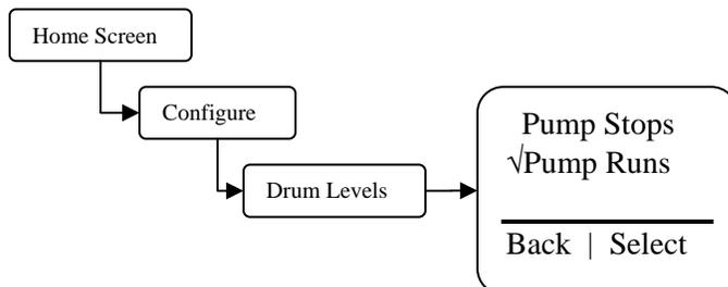
**Pump Stops** – Selecting this mode causes the inhibitor, biocide A, or biocide B outputs to de-energize when their drum level goes low.
