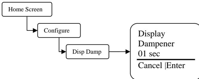
**Display Dampener** – Set this value to the number of seconds you want the controller to dampen the displayed conductivity and controller response.
