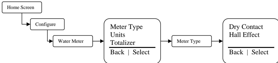
**Meter Type** – Select between a dry contact or Hall-effect water meter. Once the type is selected enter the resolution or volume per pulse.
