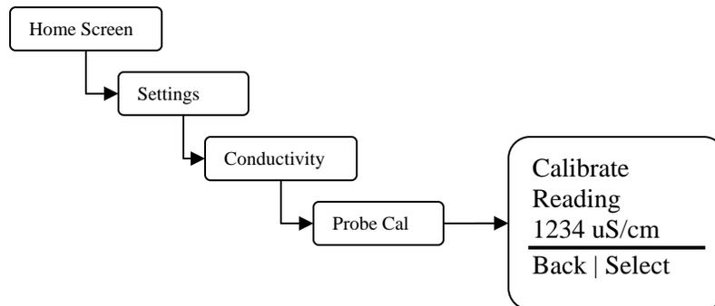
**Step 2** – Draw a sample of the process flow water and measure the conductivity using a calibrated meter. Be certain the meter you are using to measure conductivity is temperature compensated. Write down the conductivity value and sample temperature.
